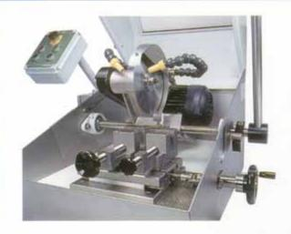
In petrographic sample preparation, cutting is the first operation to reduce their dimensions allowing the following processing steps.
