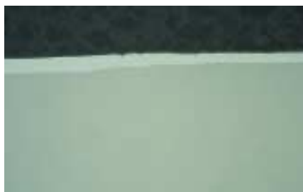
Fig.3: same as Fig.2 after 4 min. of 1 µm polish and final cleaning/polish with pure alcohol, 500x
