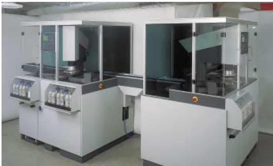
MAPS, Modular Automatic Polishing System for full-automatic preparation of large samples in high volumes, 1991
