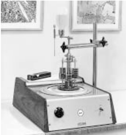
DP-4, the world's first polishing apparatus only for diamond polishing, shown with sample mover PdM-44, 1958
