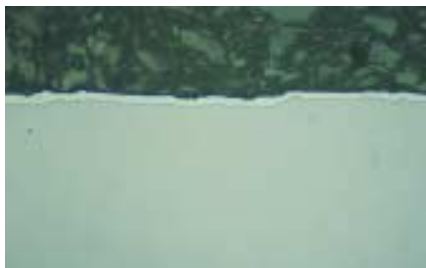
Fig. 4: Electrolytically deposited zinc coating, polished to 1 µm and final cleaning/polish with pure alcohol, 1000 x
