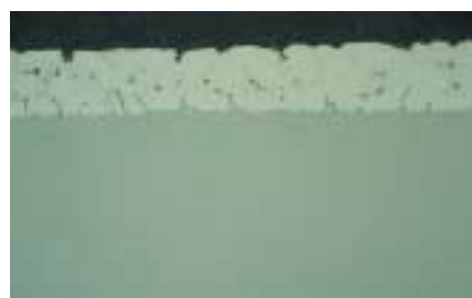
Fig. 7: Galvalum polished to 1 µm, etched with Nital, 1%, 500 x
