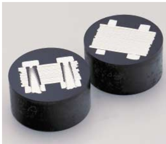
Fig. 1: Galvanized sheets in steel clamp and hot mounted
