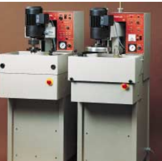
Abraplan for grinding and Abrapol for polishing, first machines in the world for "production" of materialographic samples, 1973
