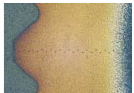
Figure 2: Detailed image of the weld seam with hardness indentations
