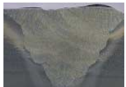
Figure 2: Detailed image of the weld seam with hardness indentations
