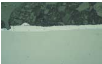
Fig. 2: Hot dip galvanized coating after 2 minutes of 1 µm polish, 500 x
