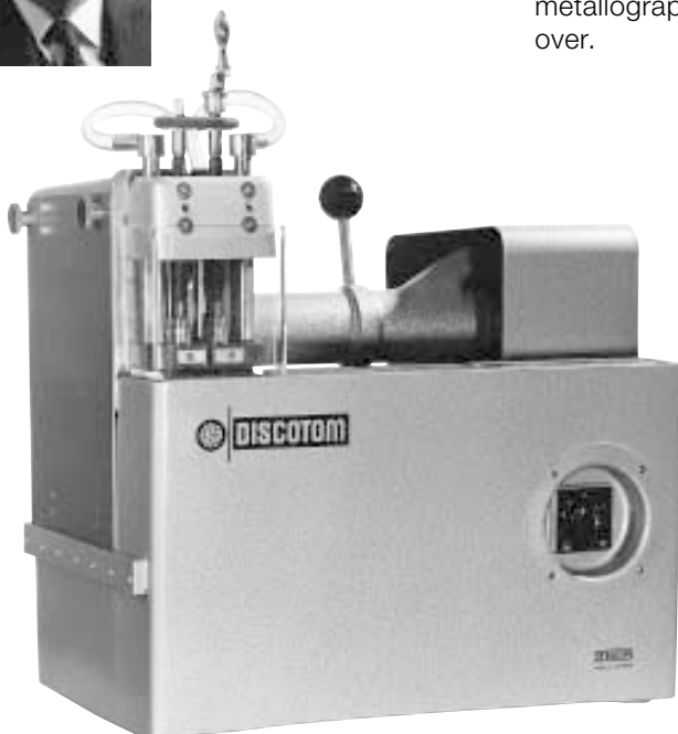
Discotom, cut-off machine, showing completely new ways of design in cutting machines, 1965
