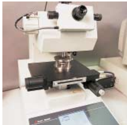
Duramin, automatic Vickers hardness tester in 4 different models, 2000
