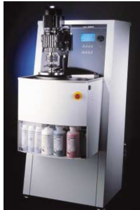
AbraPol-10, grinding/polishing machine for high volume preparation, 2000
