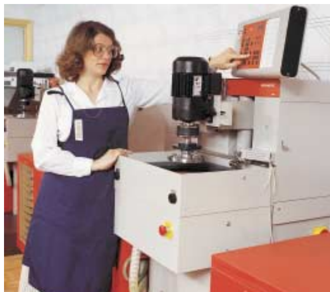
Abramatic, the world's first microprocessor controlled grinder/polisher for materialographic samples, 1983
