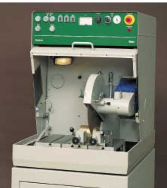
Exotom, the world's first automatic cut-off machine for materialographic samples using an oscillating cut-off wheel, 1987
