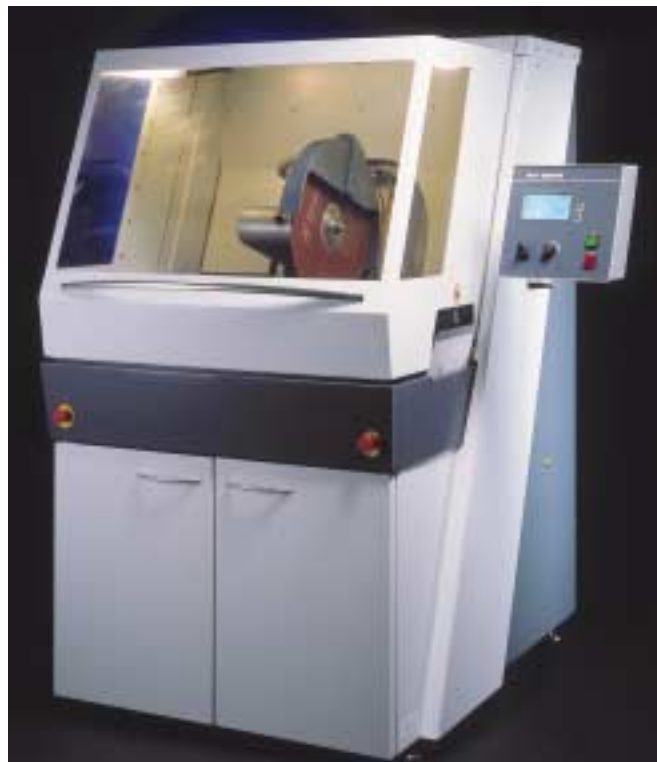
Exotom-100, cut-off machine with three different cutting modes for cutting of large workpieces of the most difficult materials, 1999
