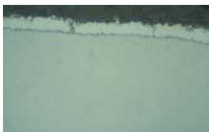
Fig. 6: Same coating as Fig. 5, etched with Nital, 1%, 1000 x
