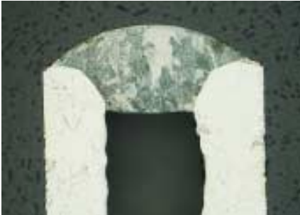
Fig. 14b Small tubes, longitudinal section, material 1.4571, (X 6 CrNiMoTi 17 12 2). Laser welded point. Dimensions 1 x 0.25 mm. Etching V 2 A-Beize
