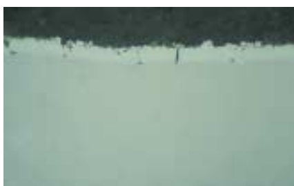
Fig. 5: Galvanealed zinc coating polished to 1 µm, 1000 x
