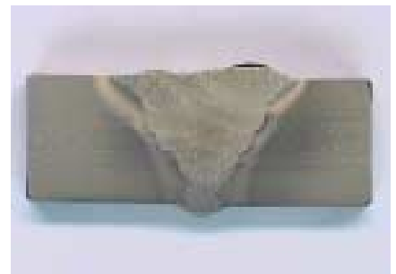
Figure 1: Low magnification image of a weld seam
