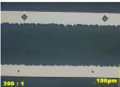
Figure 7: Detailed image of the component, indentations on the copper strip conductors
