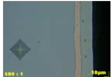
Figure 10: Indentations in the layer applied at low load. The indentation in the base material is produced using a higher load
