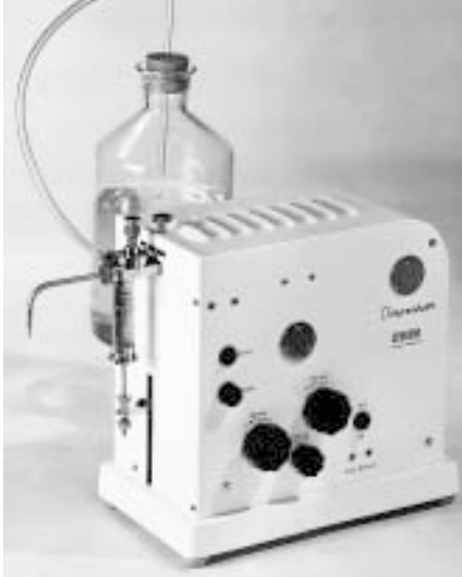
Dispenser, apparatus for exact dosing of liquids, one of the most important of the "chemical line" of products, 1952
