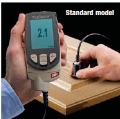
B Probe for measuring polymer coatings on wood and plastic.
